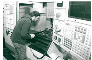
Bill Roy of Peerless Precision setting up a Haas VF3 CNC Milling machine.
